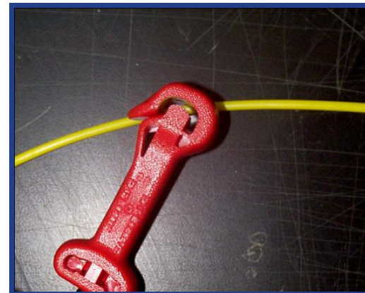
Figure 88 - Shock tube not clipped in at all.
