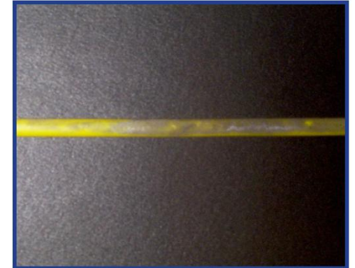
Figure 85 - Shock tube after functioning the EZ DET at left; the tube shows carbon/Al residue with no penetration marks into the jacket of the shock tube.
